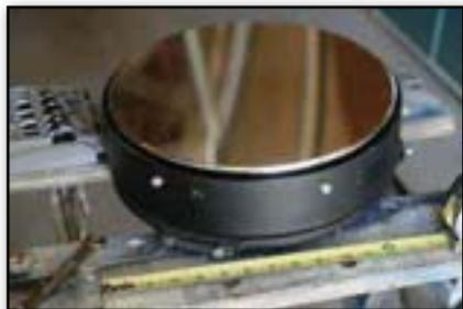
Photo at left, the mirror in the mirror cell and below left, the 2-inch focuser. The above right photo shows the secondary mirror in a spider mount.
