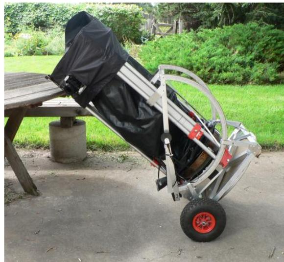
What I created is a lightweight, 50 lb., very portable, collapsible (fits in the back of my car), easy-to-collimate 12.5" mirror telescope that can be left out in the weather. Its length can be easily adjusted for my bino-viewer or my webcam, but it is mostly a fast-to-transport (with my added clip-on wheels), easy to set up, reasonable aperture, cheap aluminum telescope. It has no wood to worry about warping in the heat or cracking or delaminating. Needless to say, it's durable.
