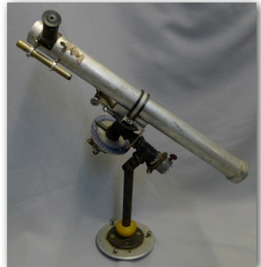
FIG. 1: THE 40MM PIPE MOUNTED NEWTONIAN, 4X10 FINDER
