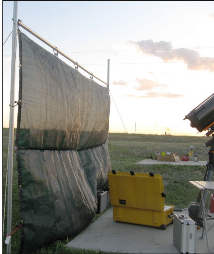
The prototype windscreen allowed accurate auto-guiding in winds up to 28 mph. The final version will have spaced hooks on the uprights to allow screen height adjustments for observing near the horizon.
