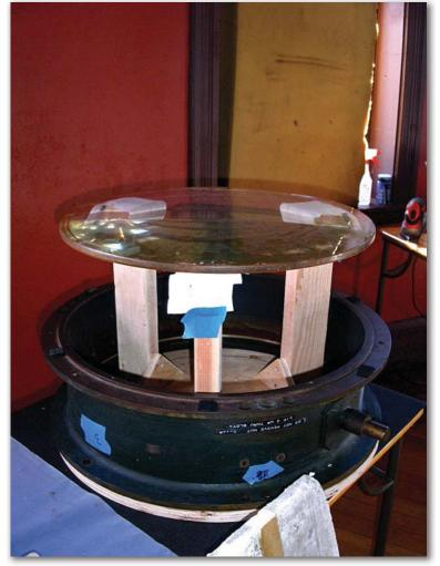
proper tooling will be needed to remove this lens. After reassembly and subsequent realignment, the numbers on the hour circle could once again be read.
