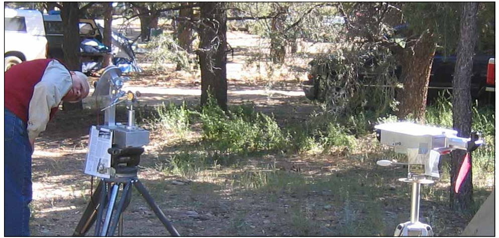
The man in the photo (not John) is examining the Heliostat mirror mechanism which tracks the sun and sends a horizontal shaft of light into the Spectroscope (on the right), where the spectrum of absorption lines are viewed through the eyepiece.
