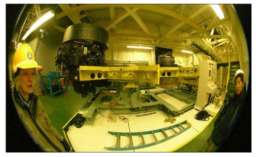
Subaru's lazy Susan for changing the focal configuration. The focal configuration changer mechanism is above the scope.
