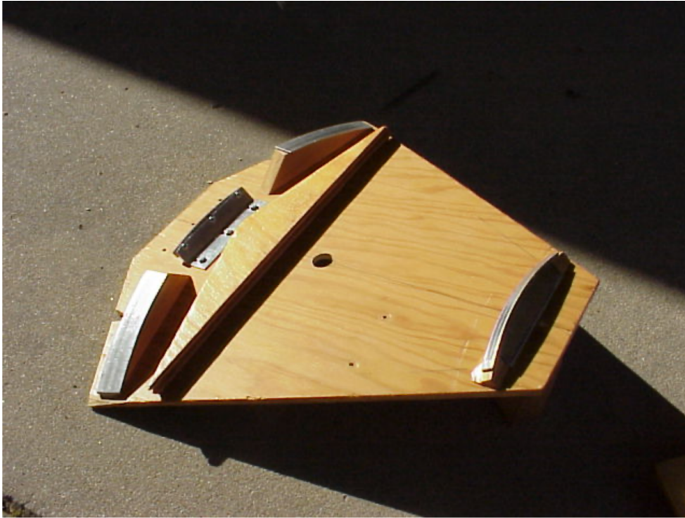
A pair of cam rollers is attached to the ground board with an angle bracket that hold the threaded insert for the adjustable feet. As the force at the roller bearing is almost vertical, only minimum support is needed from the ground board for these feet.
